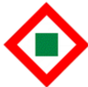
Port junction day beacon
