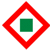
Port junction day beacon
