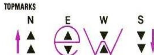
The top marks also co-ordinate with the colour scheme on the buoys. On a North cardinal buoy the top marks point up, thus the top of the buoy is black. On an East cardinal buoy the top marks point toward the ends, thus the ends are black. And on a West cardinal buoy the top marks point toward the middle, thus the middle is black. Thus, even if a buoy has been run over by a ship (breaking off the top marks) one can still identify the buoy via its paint scheme.
