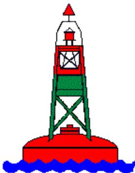
**Right-hand bifurcation buoys** (also called right-hand junction buoys) are red in colour with a green horizontal band across the midsection and are used to mark a junction where one channel splits into two. **To enter the preferred or main channel, keep a red (right) junction buoy on the starboard (right) side of your vessel when travelling upstream.**
