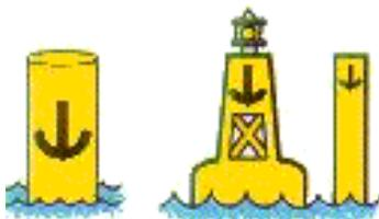
An **anchorage buoy** marks the perimeter of designated anchorage areas. One should consult the chart for anchorage depths to ensure that the anchorage can accept your vessel’s draft.
