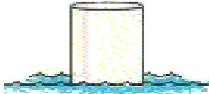
**Swimming buoys** are used to mark the perimeter of a swimming area. A swimming buoy is white in colour and carries no markings. If it carries a light, the light is yellow in colour and operates on a flash cycle, (F1) 4s, (i.e. flashing once every 4 seconds).
